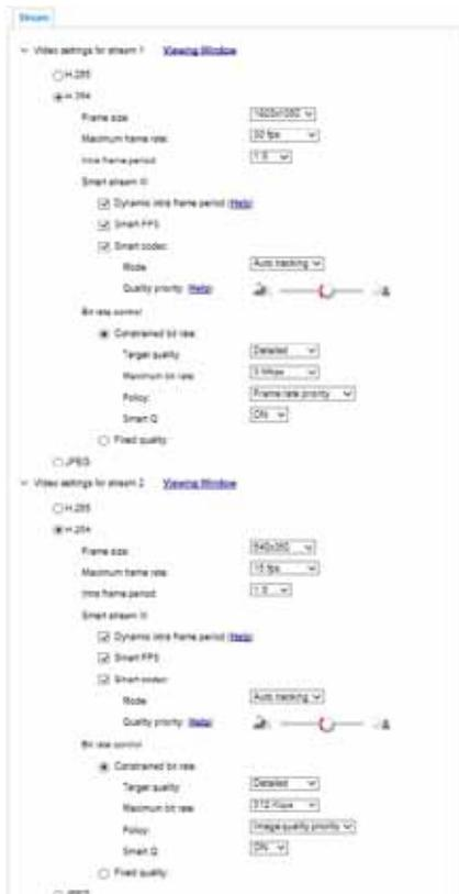
This Network Camera provides real-time H.265, H.264 and MJPEG compression standards (Triple Codec) for real-time viewing. If the **H.265** or **H.264** mode is selected, the video is streamed via RTSP protocol. There are several parameters through which you can adjust the video performance:
