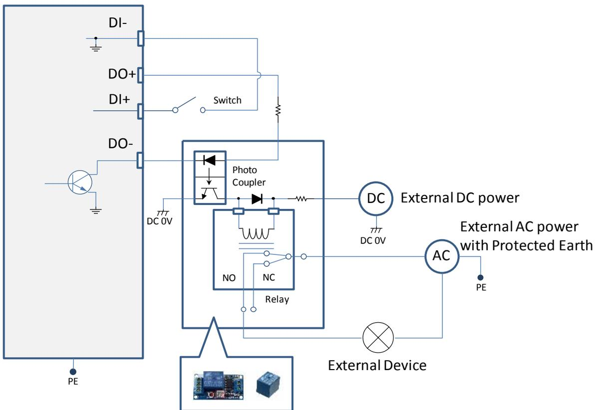
Wet contact with external DC power source to supply a relay.
