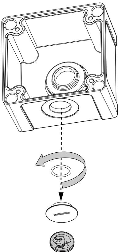
5. Route cables through the conduit, and install a 3/4" conduit to the junction box. Note that the conduit is user-supplied. Even if you route cables through the center hole, a conduit is still recommended for water-proofing.
