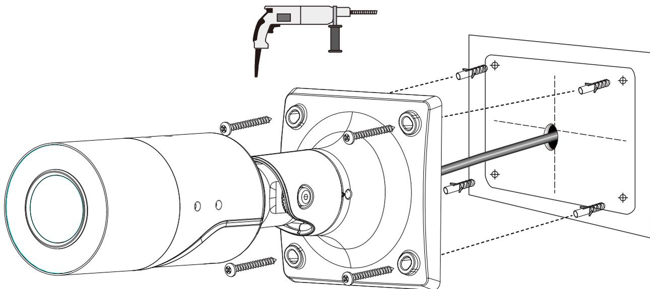
10. Use putties to seal the cable joints for water-proofing. Connect the ground wire to a grounded earth rod with a resistance smaller than  $4\Omega$ , with a section area larger than  $25\text{mm}^2$ , to a ground rod 1.5 meters into the ground.
