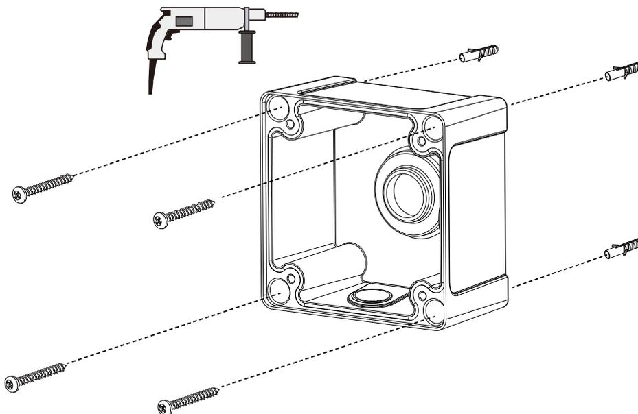
4. If you need to route cables through a conduit, remove the plastic stopper underneath the junction box.
