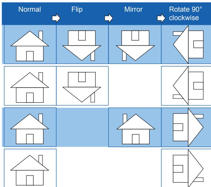
The camera may be installed on a vertical, side-facing, or tilted surface in order to accommodate the interior or exterior design of a building. The interior of a building can be shaped as a narrow rectangular space, such as a corridor. The conventional HD image, such as that of a 16:9 aspect ratio, will be incongruous with its wide horizontal view. With video rotation, the camera can more readily cover the field of view on a tall and narrow scene.
