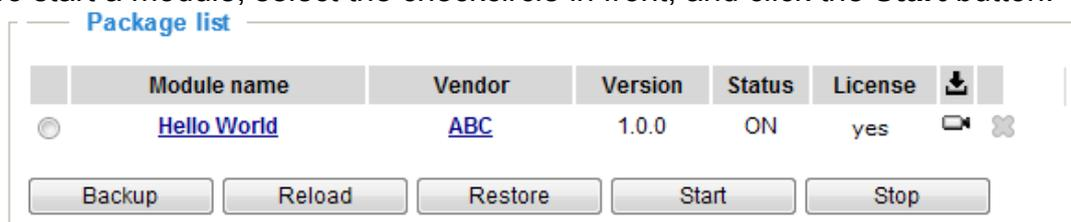
If you should need to remove a module, select the checkcircle in front and then click the **Stop** button. By then the module status will become **OFF**, and the **X** button will appear at the end of the row. Click on the **X** button to remove an existing module.
