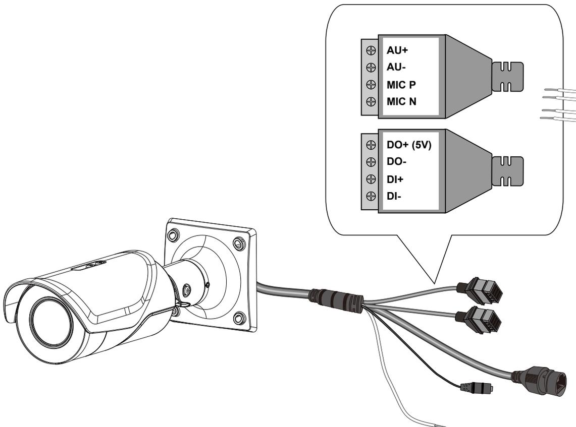
8. Pass an Ethernet cable through the waterproof cable gland components, and through the rubber seal as shown below. Connect the Ethernet cable to the camera's RJ45 onnector.
