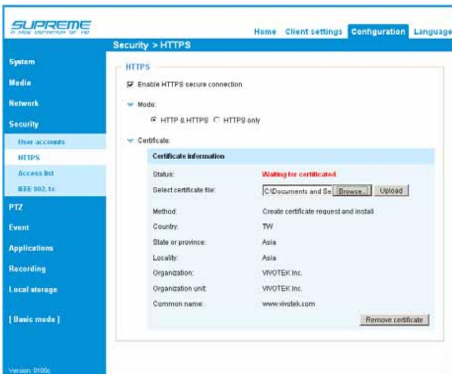
11. When the certificate file is successfully loaded, its status will be stated as **Active**. Note that a certificate must have been created and installed before you can click on the **“Save”** button for the configuration to take effect.
