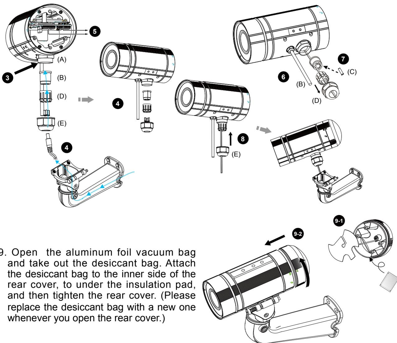
9. Open the aluminum foil vacuum bag and take out the desiccant bag. Attach the desiccant bag to the inner side of the rear cover, to under the insulation pad, and then tighten the rear cover. (Please replace the desiccant bag with a new one whenever you open the rear cover.)
