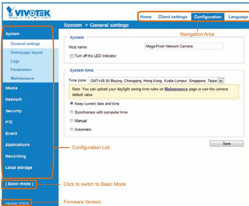
Each function on the configuration list will be explained in the following sections. Those functions that are displayed only in Advanced Mode are tagged with **Advanced Mode**. If you want to set up advanced functions, please click **[Advanced Mode]** on the bottom of the configuration list to quickly switch over.
