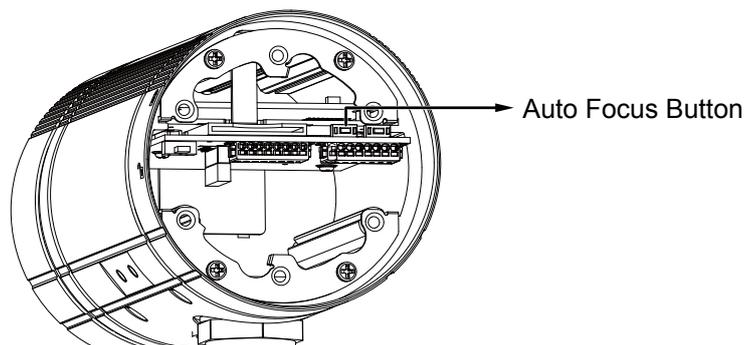
Press the button, and the camera firmware will automatically perform an auto-sensing process on its vari-focal lens to look for the best focus. The process takes about a minute to complete. This function applies when you see the image is out of focus when the surrounding lighting condition is changed drastically for some reasons. You can press the button for longer than 1 second to perform a full-range scan. Forcing a re-focusing may improve the image quality.
