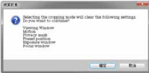
Note that the changes in cropping setting will erase the previous setting with Viewing window, motion detection, privacy mask, preset positions, etc.
