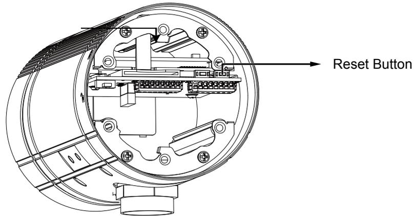
The reset button is used to reset the system or restore the factory default settings. Sometimes resetting the system can return the camera to normal operation. If the system problems remain after reset, restore the factory settings and install again.
