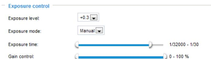
**Auto:** If you set Exposure mode as **Auto**, the Exposure time and Gain control will not be configurable since the sensor library will automatically adjust the value according to the ambient light. Then you can configure iris mode as “indoor” or “outdoor” to reach the best image quality.
