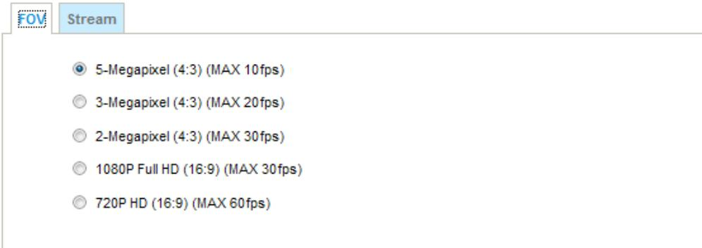
Select a resolution from the list. The default is 5 Megapixels, and if bandwidth or frame rate per second is of the concern you can select a lower resolution. The configurable options are: 5MP (4:3) at 10fps, 3MP (4:3) 20fps, 2MP (4:3) 30fps, 1080P (16:9) 30fps, and 720P (16:9) at 60fps.
