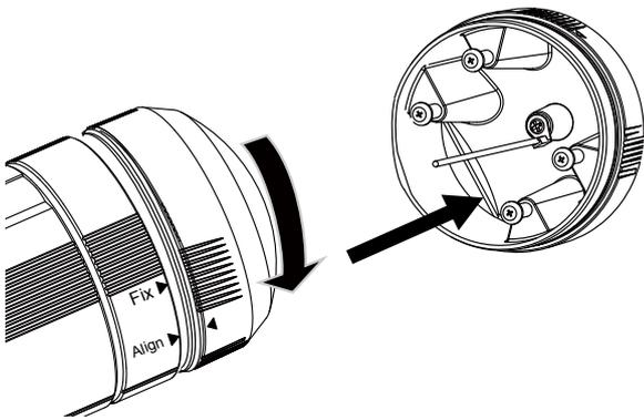
Open the rear cover by rotating to the alignment mark, and pull the cover off the canister.
