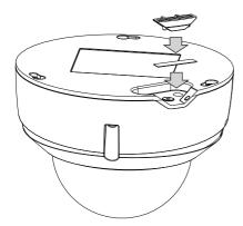
3-1-2. Refer to the camera's Quick Installation Guide for how to make the waterproof connections. Install the camera to the mounting cap by turning it counter-clockwise so that the screw heads fit in the keyhole slots. Fasten the screws, and then connect the cables.
