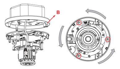
3-2-3. Tune and focus, and refer to the documentation that came with your cameras for the rest of configuration details. Install the dome cover.
