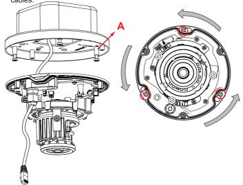
3-1-3. Tune the focus, and refer to the documentation that came with your cameras for the rest of configuration details. Install the dome cover.
