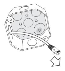
2. Install the mount cap to the junction box. Use screw holes specified on page 3 depending on the type of junction box.
