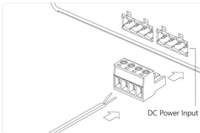
1. Pull out the 4-pin terminal block.
